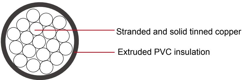
Conductor: Stranded and solid tinned copper conductor
